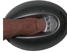
Correct (covering all of sensor)
