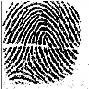
Example 5. Reasonable finger image. Not filling whole sensor image (lower corners) indicating slightly more pressure should be used. Note the naturally-occurring crease across the centre of the image.
